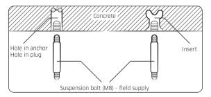
**3** Install the suspension bolts depending on the ceiling type.
